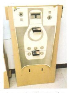
simple button will rotate between the different training programs, view, scroll and toggle between 'split time' and 'total time' performance results, set automatic or manual 'restart, choose 'random' or define the delay time for the 'start signal, define needed 'hits' on target, set training program length, set preferred sound and light response, extend targets range, define subgroups, and more...
